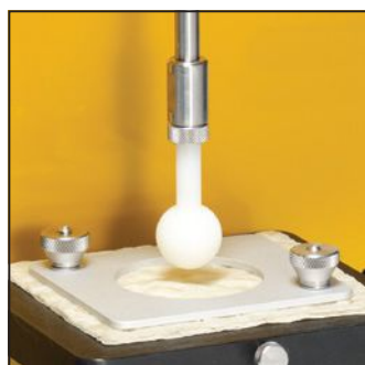
TA-DE F Dough Extensibility Fixture for holding sheet of raw dough or flat bread to measure breaking point of stretched sample. Fixture Base Table required.
