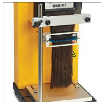
TA-HCF C Hair Combability Fixture measures the effect of hair dye, shampoos and conditioners on the combability of hair.
