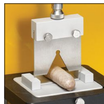
TA-SBA-WB-1 F 1mm Shear Blades for cutting-shear test: meat, fish, sausage, etc. TA-SBA-WB-3 option for 3mm blades. Fixture Base Table required.
