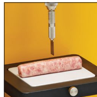
TA-52 MOHRS F Shear Blade used for cutting tests, especially meat, poultry, fish or similar products. Fixture or rotary base table recommended.
