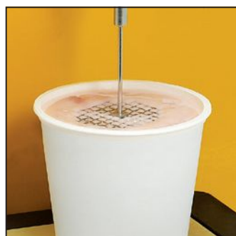
TA-MP F M Mesh Probe quantifies the consistency of products such as mayonnaise and yogurt.
