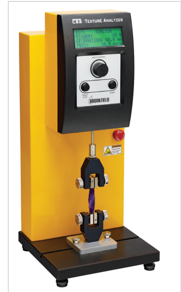
Figures 1: Brookfield CT3 Texture Analyzer with Dual Grips for Tension Test on Packaging Seal
