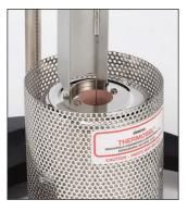
Alignment Bracket ensures concentricity of spindle and sample chamber.
