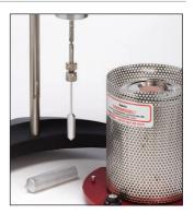
Option: Disposable Sample Chamber with Optional Disposable Spindle SC4-27D\* is ideal for asphalts or any difficult-to-clean material. Order disposable SC4-27D spindle in quantities of 100, Part No. SC4-27D-100. Requires special chuck/closer, Part No. SC4-DSY, for attachment to viscometer. Order disposable HT-2DB chambers in quantities of 100, Part No. HT-2DB-100.
