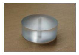
The angled taper of the test probe facilitates product flow and reduces the amount of air-pockets between the probe and sample interface. This helps with the measurement of adhesive characteristics and the movement of particulates between probe perimeter and container.
