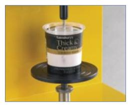
The semi-solid yogurt sample is evaluated in its commercial container. The specially-designed probe is driven into the sample under controlled conditions and a volume of product is displaced. The energy input by the Texture Analyser and the hardness of the sample are key indicators of yogurt quality.
